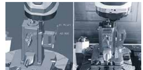
Direct connection with fixed C axis with no safety distance.
